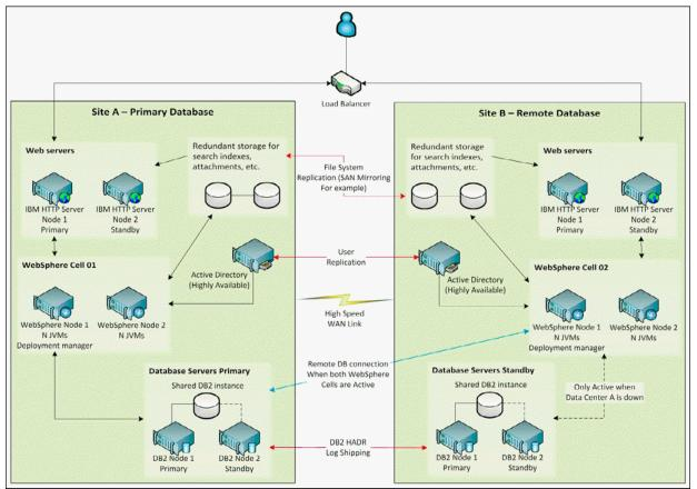
Figure 2 shows a hybrid-active topology with a remote database connection.
