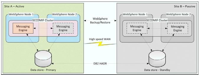
Figure 4. Service Integration Bus Active/Passive configuration
