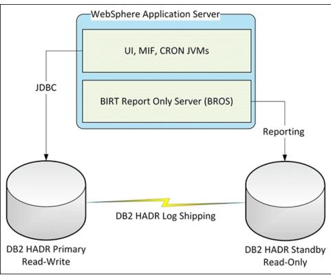
Figure 3. DB2 HADR configuration with a read-only replica
